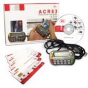
ACR83 PINeasy is a USB reader featuring a keypad and display, supporting Secure PIN Entry (SPE). The PIN (Personal Identification Number) is entered on its keypad securely and then authenticated within the device. Since the PIN is entered into the secure ACR83 PINeasy rather than the vulnerable PC or workstation, the possibility that a Virus/Trojan or USB Sniffer gets hold of the PIN is eliminated.
