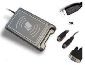
The ACR120 is a compact and cost-effective contactless reader and writer. It is developed on the 13.56MHz contactless smart card (RFID) technology, supporting Mifare® (Classics, DESFire), ISO 14443 A and B cards. Its proximity operating distance is up to 5 cm, depending on the type of contactless tag in use.
