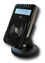
The ACR1222L is a PC-linked NFC contactless reader with LCD screen and USB host interface. Developed based on the 13.56 MHz RFID technology and the ISO/IEC 18092 NFC standard, it supports ISO 14443 Type A and B cards, Mifare, FeliCa and all four types of NFC tags.
