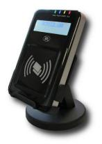
The ACR122L is a serial NFC contactless reader with LCD screen. Developed based on the 13.56 MHz RFID technology and the ISO/IEC 18092 NFC standard, it supports ISO 14443 Type A and B cards, Mifare, FeliCa and NFC technologies, including all 4 types of NFC tags and all 3 modes – reader, peer-to-peer and card emulation modes.
