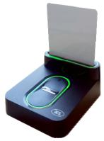
AET65 combines the core of ACS' ACR38-SAM contact smart card reader and UPEK's swipe fingerprint sensor into a single device, guaranteeing security and convenience.
